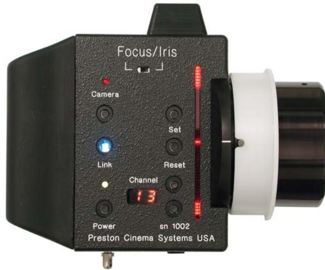
The Focus/Iris (F/I) unit is a wireless, single channel control. It can be used with the FI+Z system to take over the Iris or Focus function from the FI+Z Hand unit. When the F/I unit is powered, the FI+Z motor driver recognizes its presence and gives it control of either the Focus or Iris function of the FI+Z Hand unit as selected by the user.
